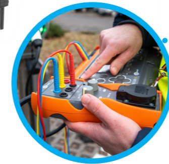
Rotary switches Quick and simple state simulation of the connected object
