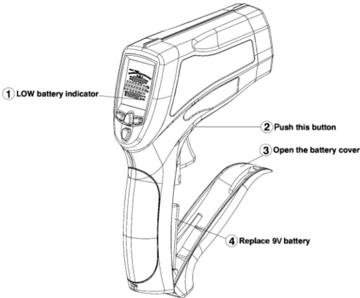
As battery power is not sufficient, LCD will display “”. Replacement with one new battery type 9V is required.
