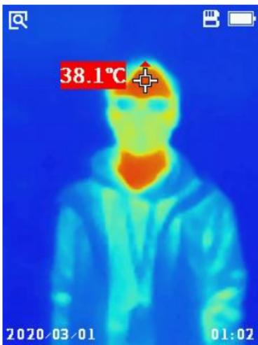
During operation of the camera, the infrared image is displayed in real time on the screen. **The temperature of the object** is displayed for the whole time.
