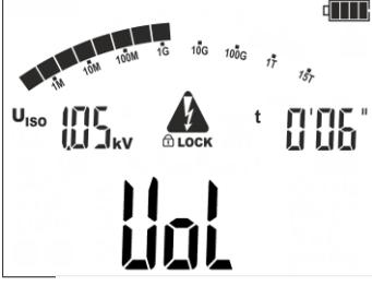
In the second phase, the device measures volume resistance  $R_{vol}$ . The screen displays message **vol** every 5 seconds.
