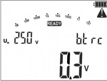
Remote control is active - **bt rc** message is displayed. A warning triangle is flashing in the corner of the screen.
