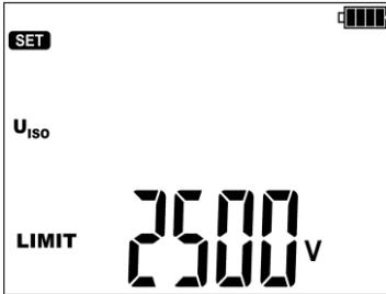
Final test voltage **U<sub>iso</sub> LIMIT**. It is within the range of 50 V...15 kV.
