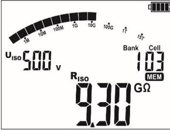
The cell is occupied by a result of the same type as the current result.
