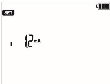
Maximum short-circuit current  $I_{sc}$  forced by the meter:
