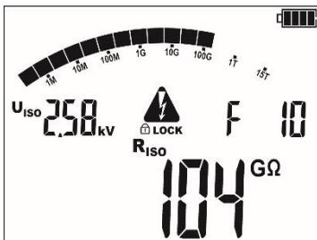
The device is equipped with an advanced **digital filter** for result stabilisation in particularly difficult and unstable measurement conditions. When the **F1** button is pressed before or during the measurement, the meter will make calculations which will stabilise the fluctuations of the test results. The meter displays a filtered value of measurements for a specified time period.
