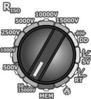
Set the rotary switch of function selection at the position of  $R_{ISO}$  measurement.
