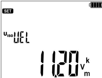
Rate of voltage increase **U<sub>iso</sub> VEL**. It is within the range of 100 V/min...12 kV/min. For example:
