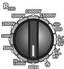
Set the rotary switch of function selection at **MEM** position.
