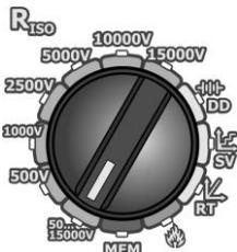
Set the rotary switch of function selection at **50...15000 V**.
