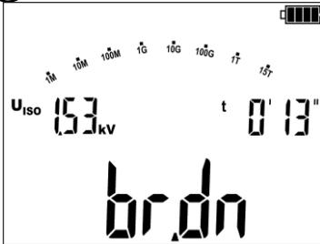
If, during the voltage increase, insulation breakdown occurs, the meter will display:
