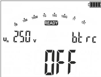
If the remote control is inactive, the attempt to initiate measurement from the mobile application produces the following message: **bt rc OFF**.
