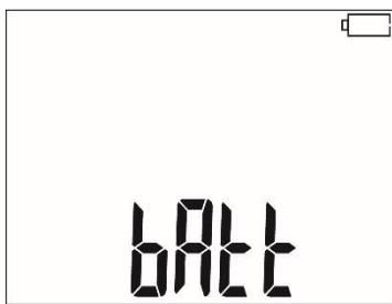
The battery is fully discharged,
