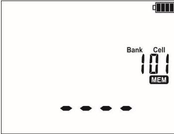
After deleting the bank, the meter beeps three times and sets the cell number as "1."
