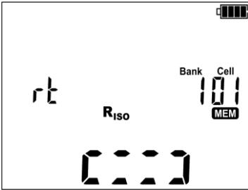
The cell is occupied by a result of a different type than the current result.
