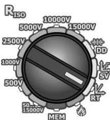
Set the rotary switch of function selection at **RT** position.
