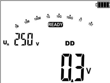
The meter is in the voltage measurement mode.
