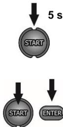
Press and hold the **START** button for **5 seconds**. This will cause 5-second countdown, after which the measurement will be **started**. Testing will be continued **until it reaches the preset time (step 6b)** or until the **ESC** button is pressed.
