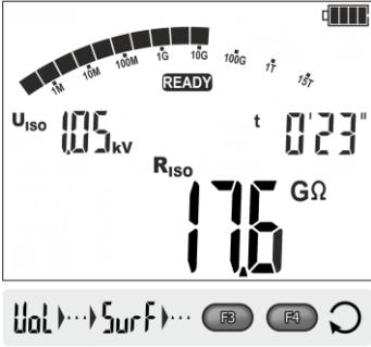
After the measurement is completed, read the results. Use the **F3** and **F4** buttons (**SCREEN**) to see individual components of the result in the following order:
