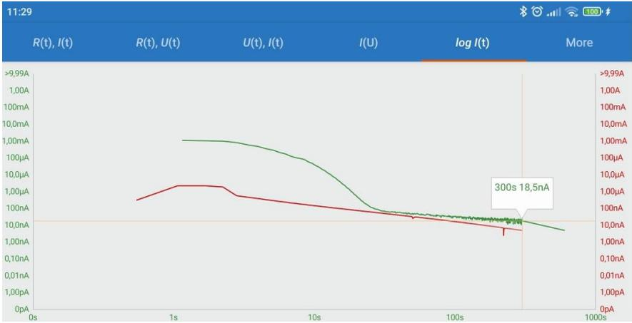
If the shape of the curves is similar, it means that the condition of the tested object is good. If the curves deviate from each other, this may indicate degradation of the insulation. Its degree can be determined by the level of difference between the curves, whereas the nature of the degradation by point of the measurement in which this difference occurred.
