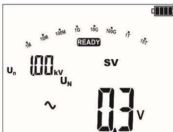
The meter is in the voltage measurement mode.
