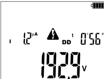
View of the screen during measurement. Phase two: object depolarization. The meter indicates:
