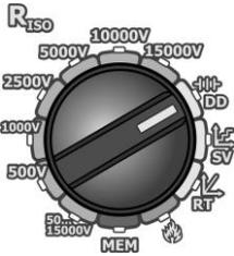
Set the rotary switch of function selection at **DD**.
