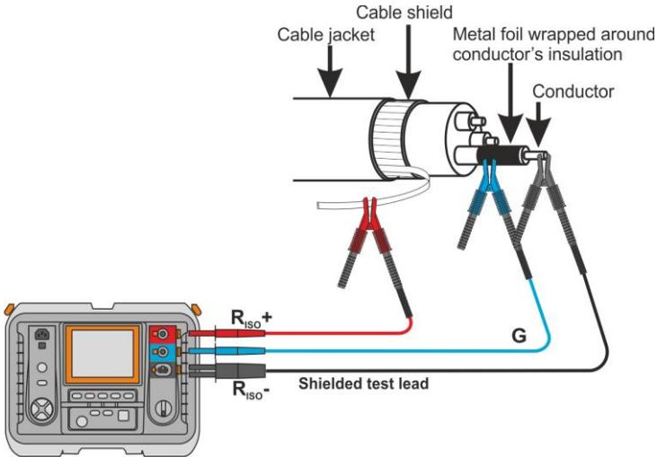
The same shall apply when measuring the insulation resistance between two conductors of the cable - other conductors that do not take part in the measurement are attached to **G** terminal.
