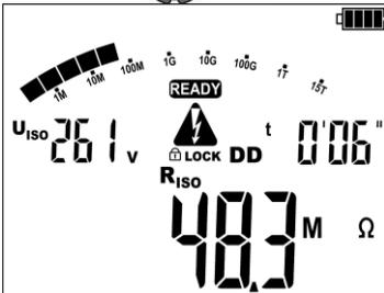
View of the screen during measurement. Phase one: object polarization. The meter indicates:
