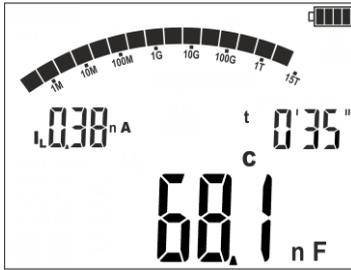
The device measures the total capacitance of the cable  $C$ . Using this value and knowing the unit capacitance  $C_x$ , the length  $L$  may be calculated.
