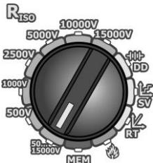
Set the rotary switch of function selection at one of  $R_{ISO}$  positions, selecting in this manner the measurement voltage.
