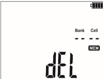
...it disappears, replaced by the symbol **dEL** signalling readiness to delete.
