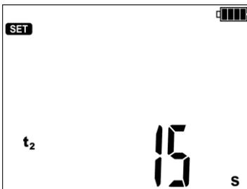
Time **t<sub>2</sub>**, for which voltage should be present on the tested object (**Graph 4.2**).
