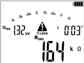
In case of insulation breakdown, the meter does not stop the measurement. The measurement lasts until the expiry of the time preset in step 3.
