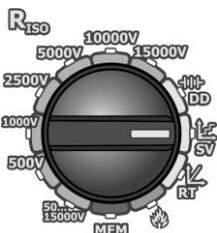
Set the rotary switch of function selection in the **SV** position.
