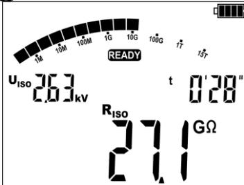
If there is no breakdown, the screen will display the values as for the measurement  $R_{iso}$ .
