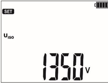
Test voltage  $U_n$  (only for positions **50...15000 V**).
