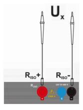
Connect the meter to a voltage source.
