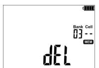
... and the cell number will change into "--", then symbol del will be displayed to indicate the readiness for deleting.
