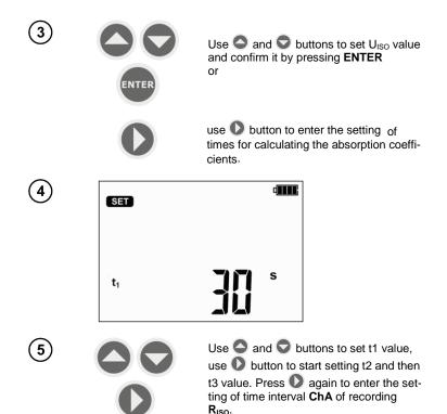
Defining ChA interval will enable the user, using Sonel Reader software, to plot the resistance chart and current chart using the data obtained from the performed measurement (see example below).
