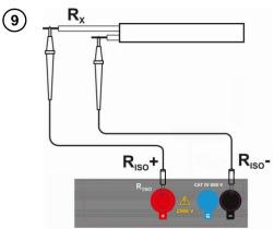
Connect test leads according to the drawing.
