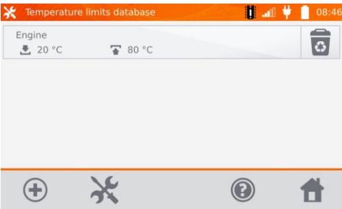
Enter and save the limits using the same method as described in section 2.3.4. Use **🗑** button to cancel the limit.
