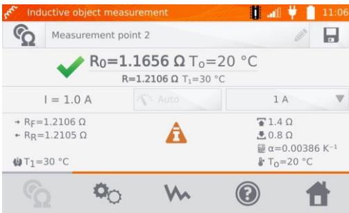
Correct result:  $R_{PE}$  within limits.
