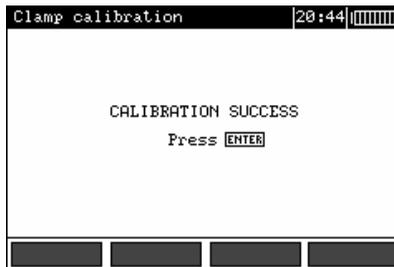
The meter has determined the correction factor for connected clamp. The factor is saved in the memory also when the power supply of the meter is off until the following successful calibration of the clamp has been performed.
