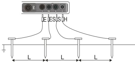
Connect the four aligned and equally spaced electrodes, which are driven into the ground, to the meter, and do so in accordance with the diagram above
