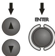
Use buttons ▲ and ▼ to set the measuring voltage and press **ENTER**.
