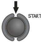
Press **START** to commence measurement. The meter will activate the mode of selection of the distance between electrodes.
