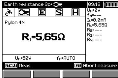
After the measurement of the first leg of the pole, the measured resistance value of the tested leg is shown on the main screen as R1 for 5 seconds. After this time, the meter transfer R1 result to the window on the right side and displays a message to the user to connect the clamps to another leg of the pole.
