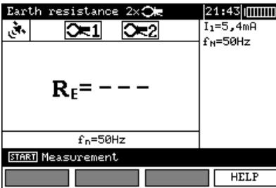
The meter is ready for measurement. The auxiliary display shows the value of the leakage current passing through the clamp and its frequency.
