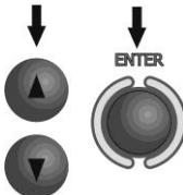
Using buttons ▲, ▼ select GPS on or off. Press **ENTER** to select the option.
