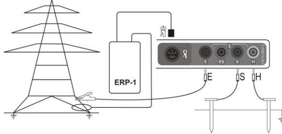
The current electrode (driven into earth) should be connected to **H** socket of the meter. The voltage electrode (driven into earth) should be connected to **S** socket of the meter. The tested leg of the pole should be connected to **E** socket of the meter with the lead. The tested leg of the pole, the current electrode and the voltage electrode should be arranged in one line. Clamps should be attached to the tested leg of the pole below the connection point of **E** lead.
