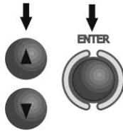
Use buttons ▲ and ▼ to set the measuring voltage and press **ENTER**.
