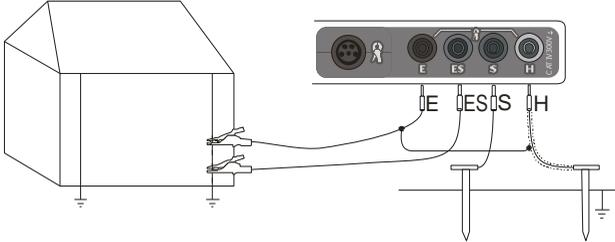
Connect the current electrode driver into ground to the **H** socket of the meter.
