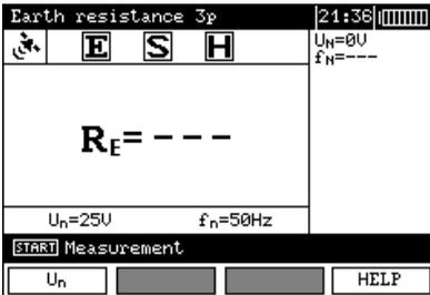
The meter is ready for measurement. The auxiliary display shows the value of the interference voltage and its frequency. The setting bar shows the mains frequency set in the MENU.
