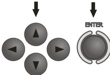
Using buttons ▲, ▼, ◀ and ▶ select the result and the distance unit and press **ENTER** to confirm.
