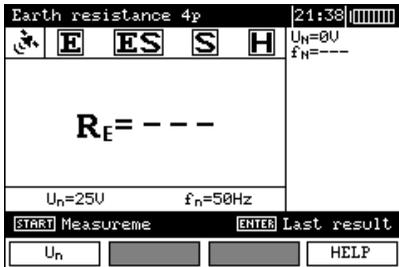
The meter is ready for measurement. The auxiliary display shows the value of the interference voltage and its frequency. The setting bar shows the mains frequency set in the MENU.
