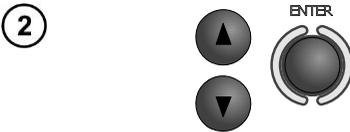
Using buttons ▲ and ▼ highlight the required position. Press **ENTER** to select the option.
