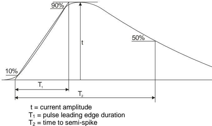
The pulse shape is determined by the relation  $T_1/T_2$  eg:  $4/10 \mu s$ .
