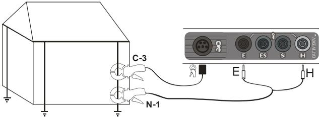
Connect the transmission clamp to sockets **H** and **E**, while the measurements clamp should be connected to the clamp socket. Snap the transmission clamp and measurement clamp on the tested earth electrode AT east 30 cm from each other.
