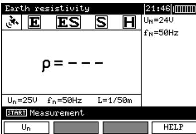
The meter is ready for measurement. The auxiliary display shows the value of the interference voltage and its frequency. The setting bar shows the measurement voltage, mains frequency set in the **MENU** and the distance between the electrodes.
