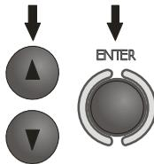
Use buttons ▲ and ▼ to select **Battery discharging**, and press **ENTER**.
