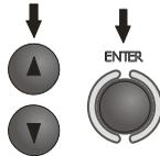
Use buttons ▲ and ▼ to set the distance between electrodes and press **ENTER** in order to commence measurement.
