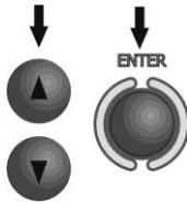
Use ▲, ▼ buttons to select the measurement with ERP-1, press **ENTER**.
