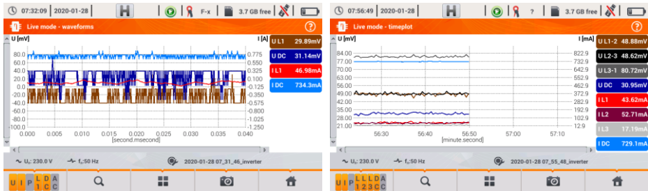
Fig. 48. Screens for waveforms and timeplots in the mode of inverter efficiency measurement
