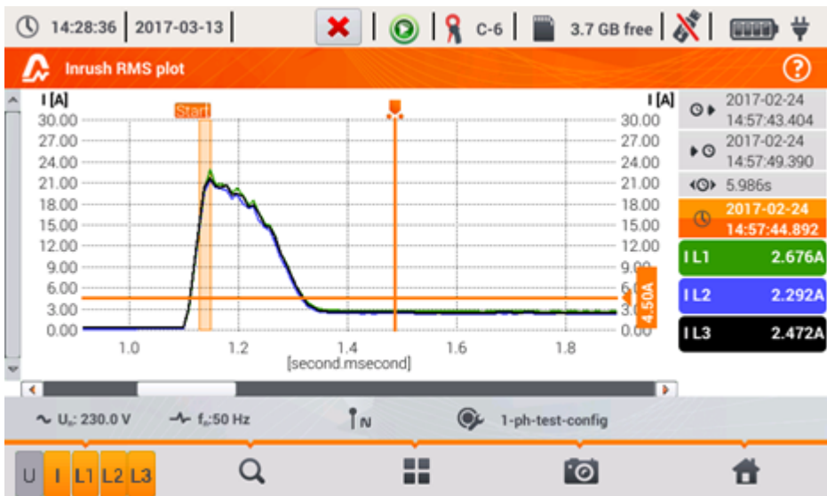
Fig. 43. Inrush current analysis – Inrush RMS plot.
