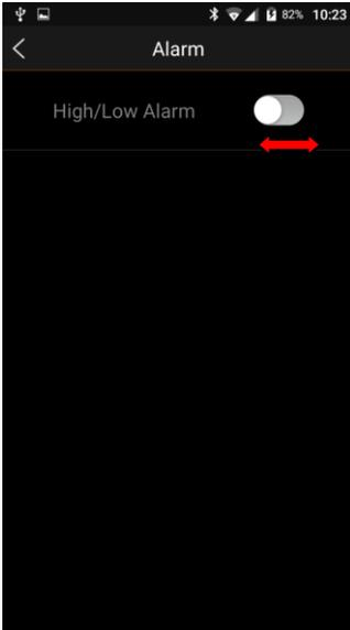
The user may set the **measuring range**. Each readout outside of the range will trigger the alarm.
