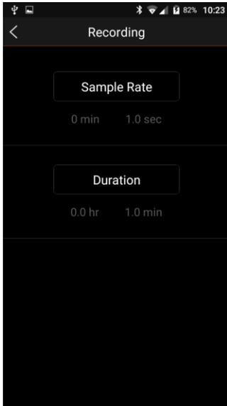
This screen allows user to modify the parameters of recording the measured quantity waveforms. Available options:
