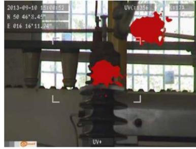
*Fig. 3, 4. Corona discharge in laboratory conditions.*
