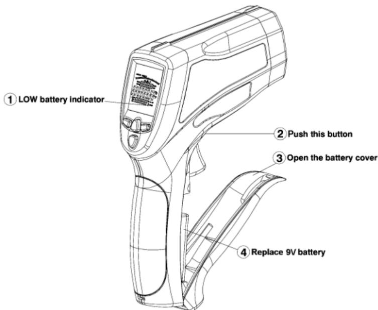
As battery power is not sufficient, LCD will display “
