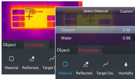
Select **Material** to change measured object's emissivity:
