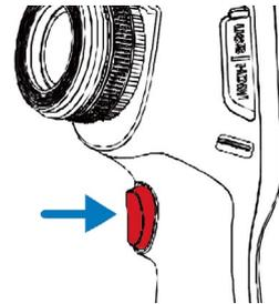
Press trigger to start/stop recording.
