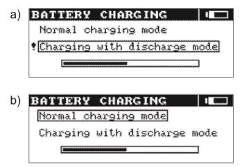
After approximately 5 seconds (the time is roughly indicated by the progress bar) the meter automatically passes to the charging mode indicated with a frame. In order to change the charging mode, proceed as follows:
