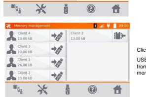
Click 1/2, to save data in the USB stick or the to copy data from the USB stick to the memory of the meter.
