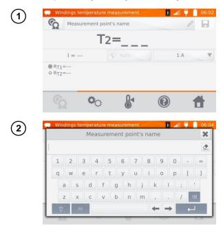
When necessary, name the measuring point.
