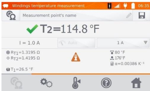
$R_{T1}$  – resistance of the cold winding
