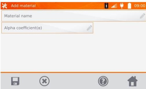
Enter and save the material and  $\alpha$  coefficient, using the same method as described in section 2.3.4.
