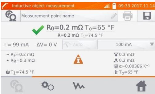
Correct result:  $R_{PE}$  within limits.
