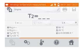
Connect the meter to the motor windings. Press START/STOP.
