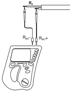
Connect test leads according to the drawing.
