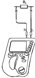
Connect the test leads as shown on the drawing.
