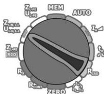
Turn the rotary switch to one of the loop impedance measurement ranges.
