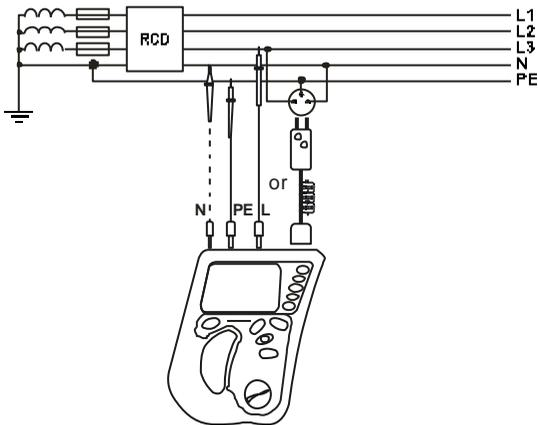
Connect test leads according to the drawing.
