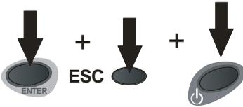
Turn on the meter, holding **ENTER** and **ESC** buttons pressed.
