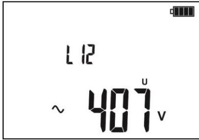
After a few seconds or after pressing **ESC** button, the meter returns to displaying the phase sequence.
