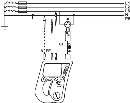
Connect the test leads according to one of the drawings.
