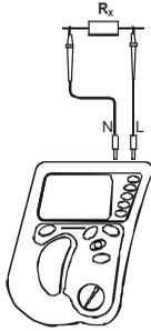
Connect the test leads according to the drawing, the measurement starts automatically.
