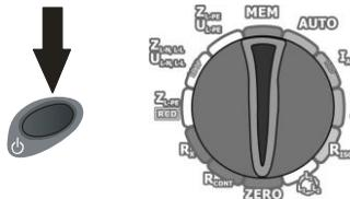
Turn on the meter. Turn the rotary switch to **ZERO** position.
