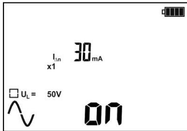
After each activation turn-on tested RCD.
