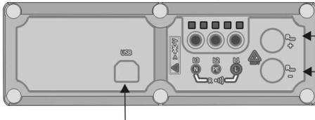
High voltage converter output for insulation resistance measurements.
