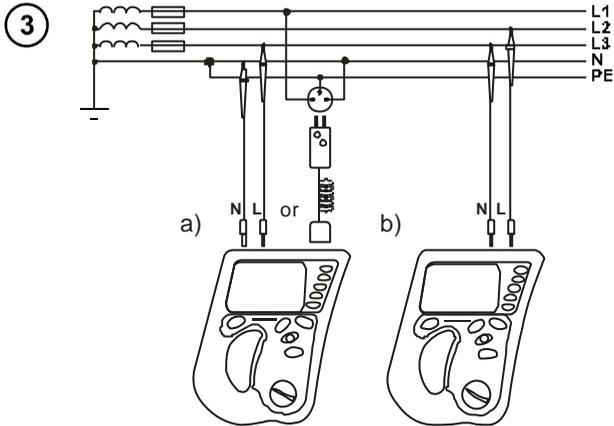
Connect test leads according to the drawing
