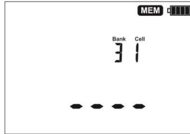
The deletion progress is shown on the display in %. When deletion is complete, the meter generates three short beeps and sets the cell number to 1.
