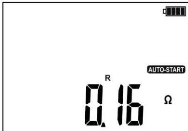
Read the main measurement result which is the arithmetic mean of two measurements with 200mA current flowing in opposite directions.
