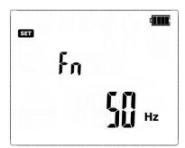
After switching the meter ON, a screen is shown with network frequency settings **Fn**.
