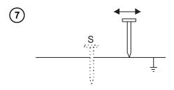
Repeat the measurements (steps 4, 5, 6) moving the voltage electrode a few meters - placing it farther and closer to the measured earth electrode.
