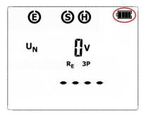
The charge level of the batteries or rechargeable batteries is indicated by the symbol in the right upper corner of the display on a current basis:
