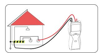
Test leads should be connected to the measurement terminals in the device, as shown above.
