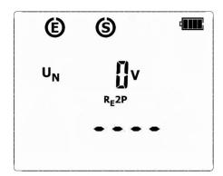
In measuring functions, before **START** button is pressed, the meter monitors the measuring voltage at the terminals (between **E** socket and **S** / **H** sockets) and the interference voltage value is displayed on the screen.
