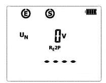
The meter is in the mode of measuring the interference voltage between the test terminals. The measuring voltage is compatible with the voltage selected when setting up the device.
