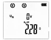
After the measurement, its result is shown: at the bottom of the screen, the main result is shown for R<sub>E</sub>2P, whereas the upper part of the screen shows the measured interference voltage U<sub>N</sub>. The result is displayed for 20 seconds. The result can be recalled by pressing UP button.
