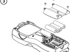
Remove the screws that secure the battery cover at the bottom of the compartment(4 pcs),
