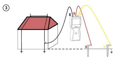
Test leads should be connected to the measurement terminals in the device, as shown above.
