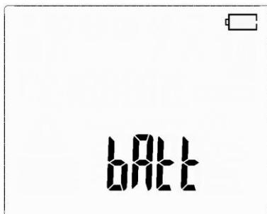
Rechargeable batteries completely discharged.
