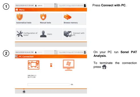
There is also a possibility to manage the meter (settings, auto procedures etc.) using **Sonel Reader** software. To do so:
