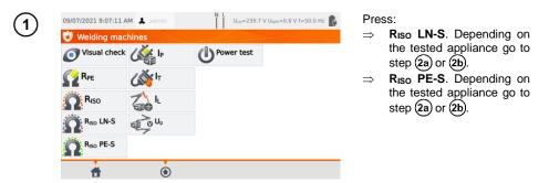
Before starting the measurement, similarly to sec. 4.2, following parameters must be set: test voltage U<sub>ISO</sub>, test duration and limit.
