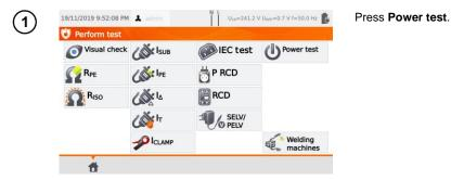
Before starting the measurement, similarly to **sec. 4.2**, following parameters must be set: **test duration** and **clamp**.
