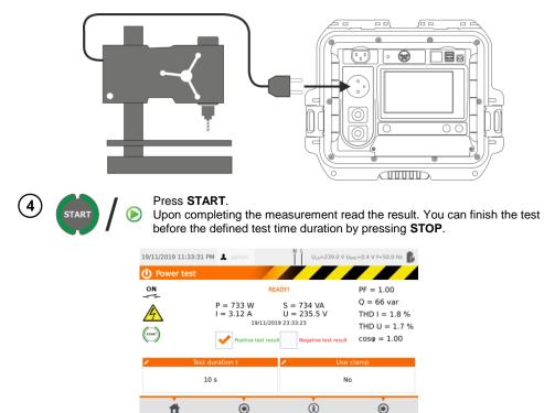
Compare the result with the technical data of the tested appliance. The assessment of the correctness of the test results can be performed by selecting the proper field in '**Positive test result**' or '**Negative test result**'. When saving test results in the memory, this assessment will also be saved along with the results.
