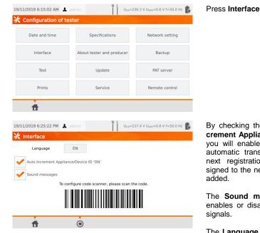
By checking the box **Auto Increment Appliance/Device ID**, you will enable or disable the automatic transmission of the next registration number assigned to the next device being added.
