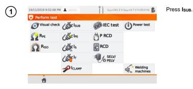
Before starting the measurement, similarly to **sec. 4.2**, following parameters must be set: **test duration** and **limit**.
