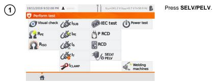
Before starting the measurement, similarly to **sec. 4.2**, following parameters must be set: **test duration** and **limits**: lower and upper.
