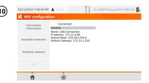
The **LAN** field displays a screen containing meter's IP in a situation, when it is connected to a LAN network.
