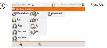
Before starting the measurement, similarly to **sec.4.2**, set  $U_0$  voltage, **secondary voltage** type, **limit PEAK**, **limit RMS** and optionally also the criterion of ±15% PEAK.
