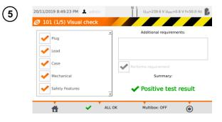
After visual test, check (or not) the corresponding boxes on the left side of the screen.
