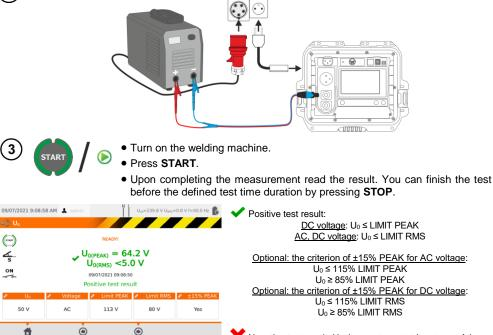
$\mathbf{X}$  Negative test result: U<sub>0</sub> does not meet at least one of the above conditions.
