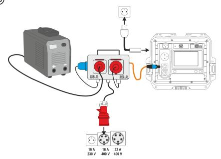
Measurement with PAT-3F-PE adapter. Connecting a 3-phase 32 A appliance.
