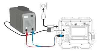
Measurement of R<sub>ISO</sub> LN-S or R<sub>ISO</sub> PE-S. 3-phase appliance or 1-phase appliance powered by an industrial socket.
