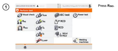
Before starting the measurement, similarly to **sec. 4.2**, following parameters must be set: **test volt-age**, **test duration**, **limit** and test method: **probe-socket** (measurement between shorted L-N and PE of the test socket or T2 probe), **probe-probe** (measurement between T1 and T2 probes) or **IEC** (IEC cord test).
