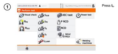
Before starting the measurement, similarly to **sec. 4.2**, following parameters must be set: **test duration, limit, polarity** and **method**.
