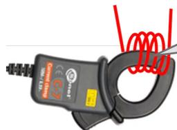
$$\text{New range} = \frac{100 \text{ A}}{5 \text{ turns}} = 20 \text{ A}$$
