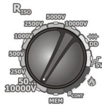
Set the function selection switch to any desired  $R_{iso}$  position. Test voltage selection: **50 ... 10,000 V** setting.
