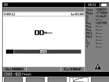
Both during and after measurement, the display can be switched back and forth between the results and the diagram by pressing **F4** .
