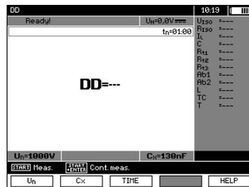
Use keys **F1** **Un**, **F2** **Cx** and **F3** **TIME** to select the desired voltage, capacitance and test time (1 to 60 min.) for the device under test. The measuring procedure is similar to the one described above in section 3.2.2.
